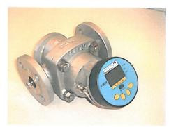
The new flow meter series (COGEM) released in 2004 and which series is operating with an electronic indicator only, does have the build in facility of linearization of the indication. COGEM can be supplied with either mentioned indicator or as blind unit with pulse output.
